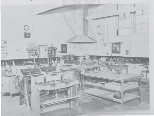
**Teacher's Demonstration Bench** (Figure 80) 32" high with a hardwood top and drawers with locks to house supplies and special tools. The bench should be equipped with both a woodworking and a metalworking vise. An electrical outlet with 110 volt current should be attached to the bench. Ideally the bench should be 30" from a blackboard at the front of the demonstration tables. A hand operated bell or other device attached to the side of the demonstration table is useful for assembling students.
