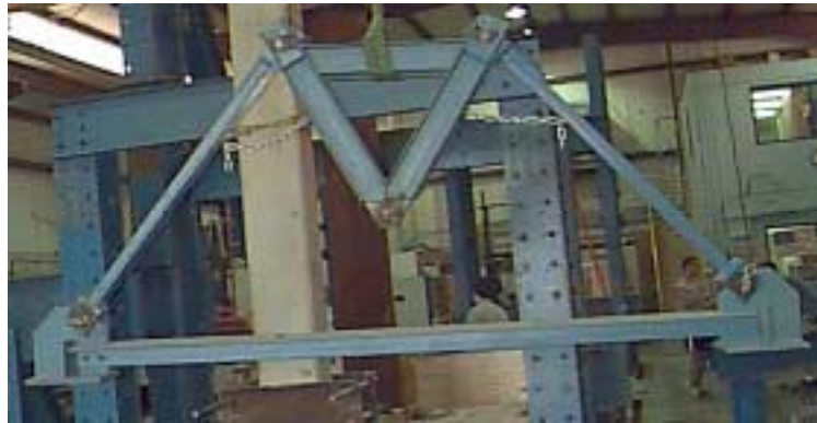
Figure 5.5. Gravity load simulator (GLS)
