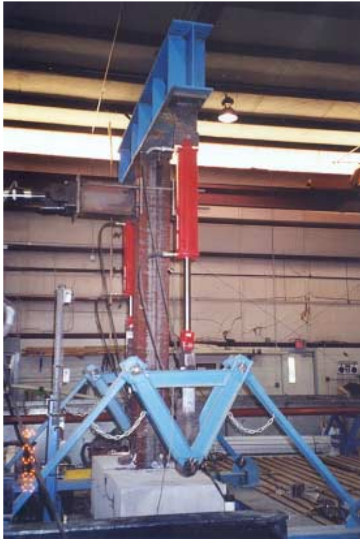
Figure 5.4. Vertical load application to piles
