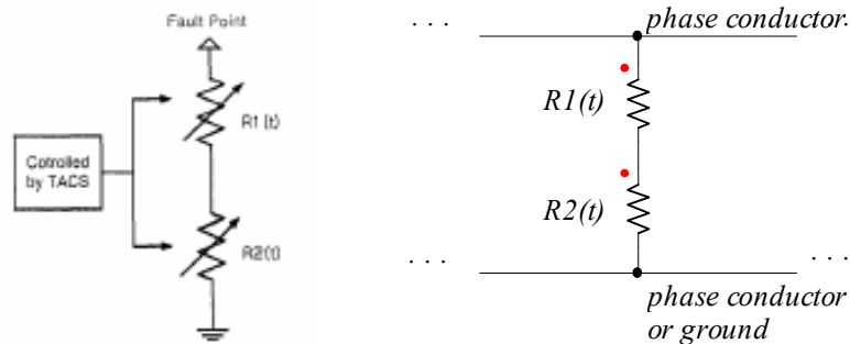
Figure 18. HIF model using two time-varying resistances (left: KEPCO’s EMTP model. Right: Simplorer®’s equivalent)
