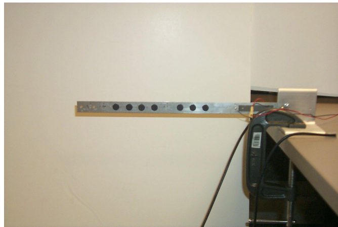
Figure 5.2 Photo of the experimental beam-mass setup.
