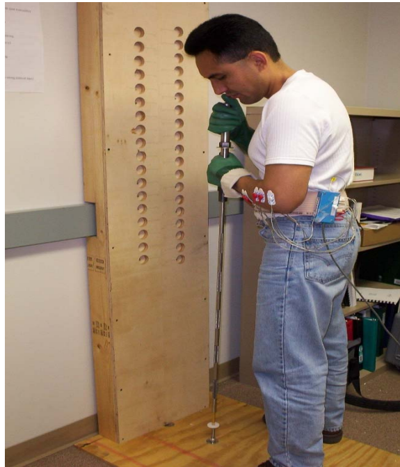
Figure 2: Participant performing condition in which the lance is parallel to the operator.
