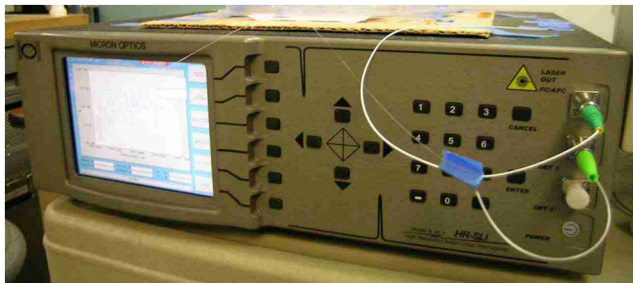
Fig. 5.7 Photo of the sensor interrogation system
