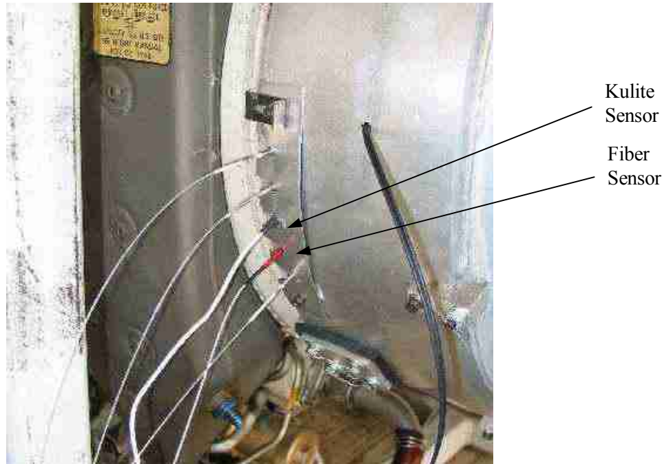
Fig. 6.26 Engine pressure sensor installation (side view)
