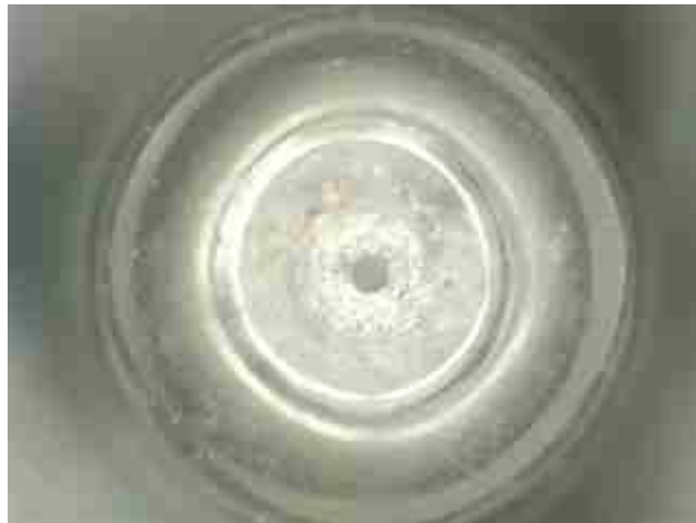
Fig. 4.11 The diaphragm to ferrule end bond (top view under microscope)
