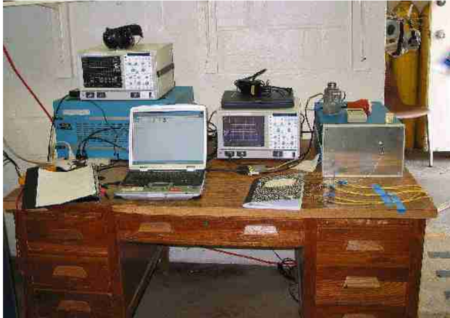
Fig. 6.28 Sensor signal processing and data acquisition devices
