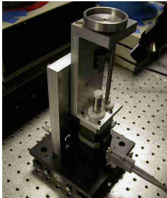
Fig. 4.9 Photo of the sensor laser bonding fixture
