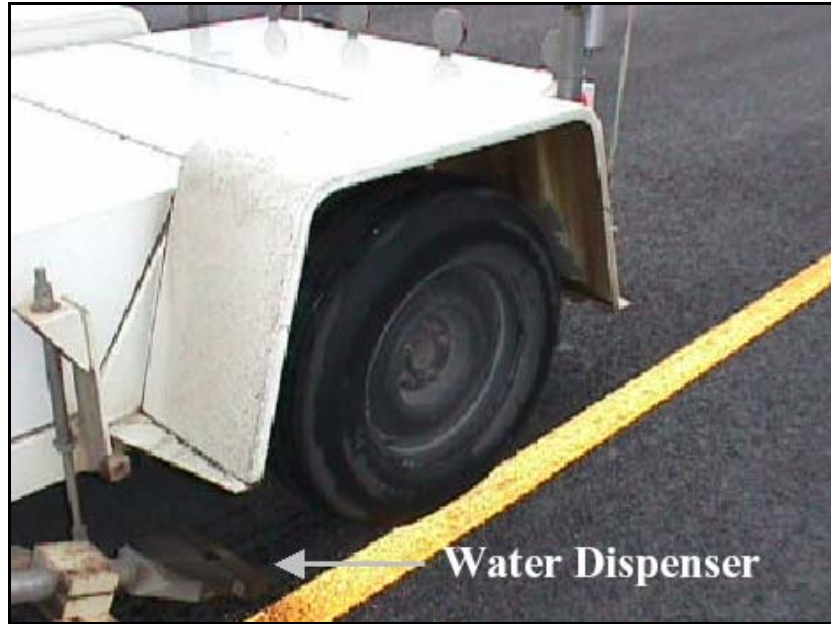
Figure 3.1 Prewetting System of Skid Trailer
