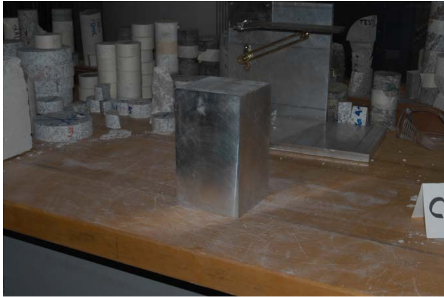
Figure 5.4: Aluminum specimen tested to detect any possible friction phenomenon internal to the testing machine.
