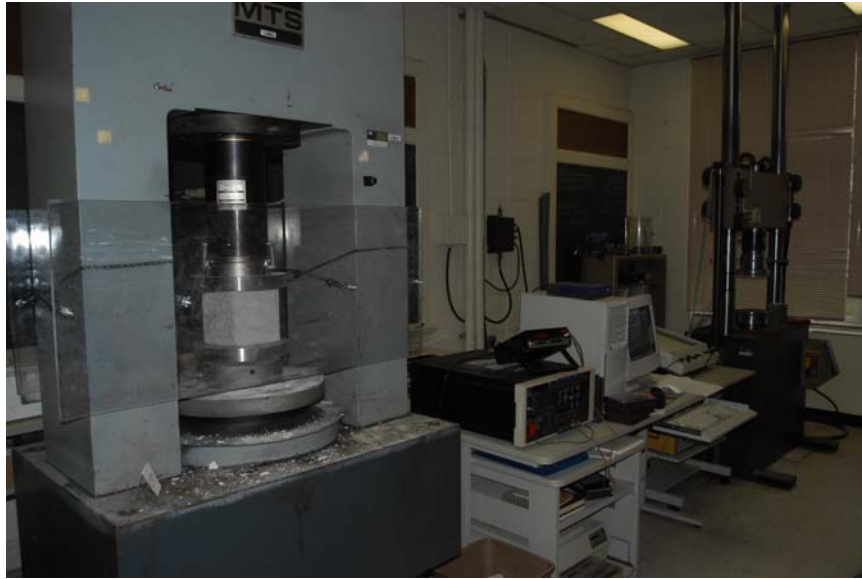
Figure 4.4: The 4448 kN MTS Machine used for ramp failure tests. The clear plastic safety shield can be seen with a specimen in place behind it.
