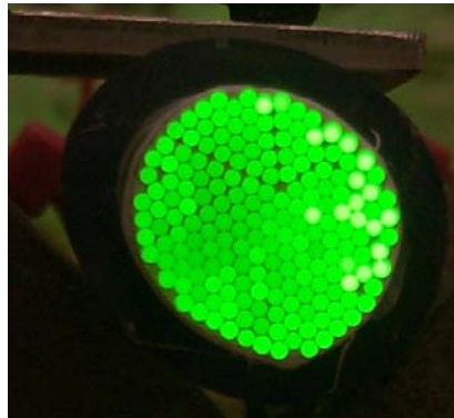
Figure 6: Picture of one end of the detector module. Room light was dimmed for the picture to emphasize the high light output of the fibers.
