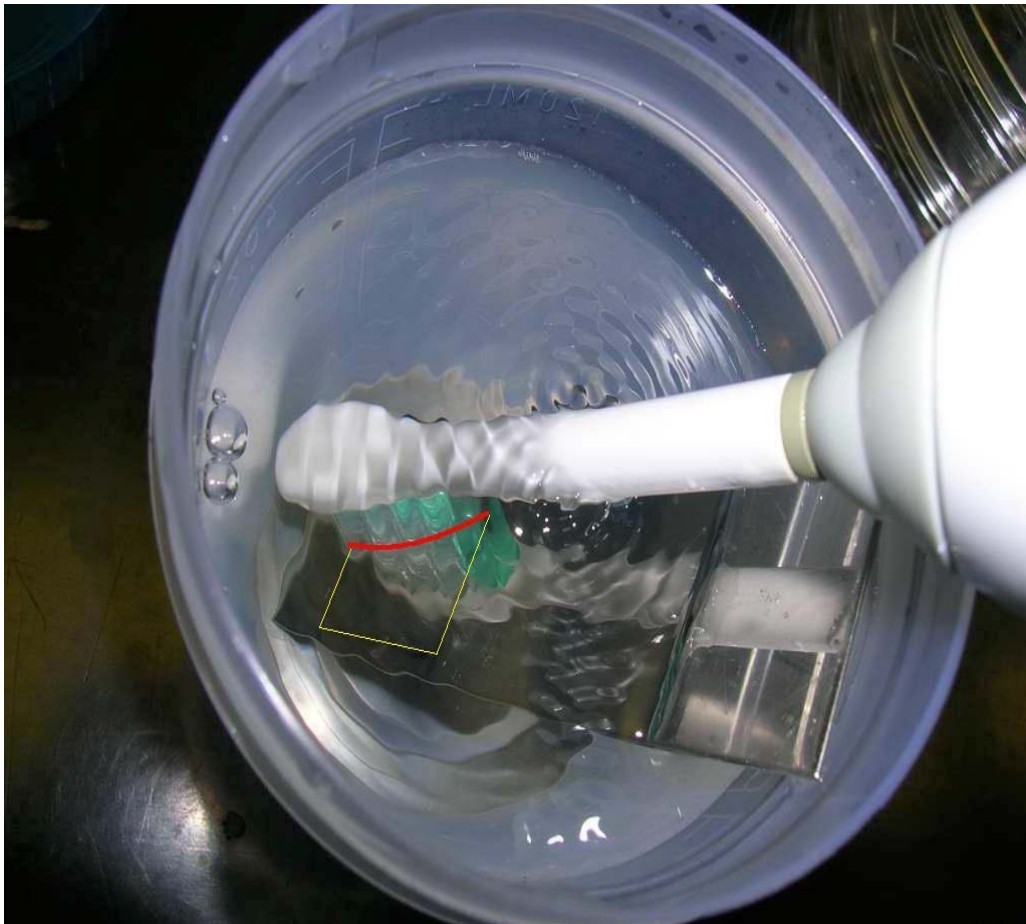
Appendix A, Figure 3: Sonicating brush head in relation to the inoculated area of the stainless steel coupon submerged in 100 mL of PBS containing 1% polysorbate 80
