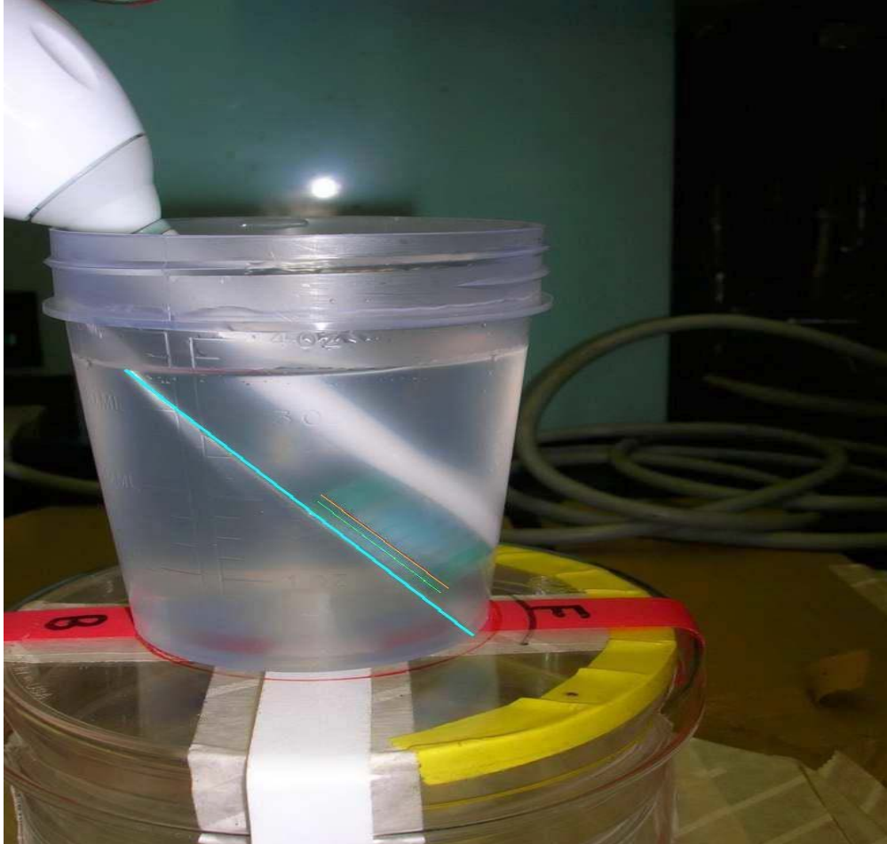
Appendix A, Figure 4. Position of sonicating brush head relative to the angle and inoculated area of the stainless steel coupon in 100 mL of PBS containing 1% polysorbate 80 during brush non-contact method.
