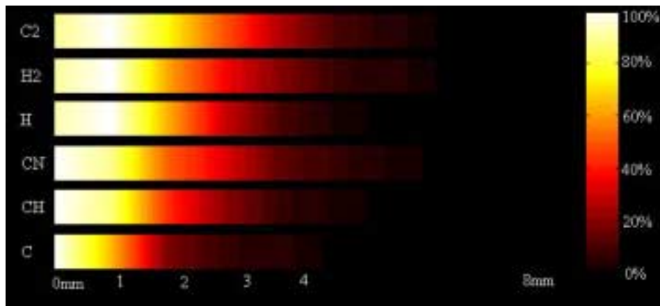
Figure 7.1: Radical Concentrations Along the Centerline of the Plasma Jet
