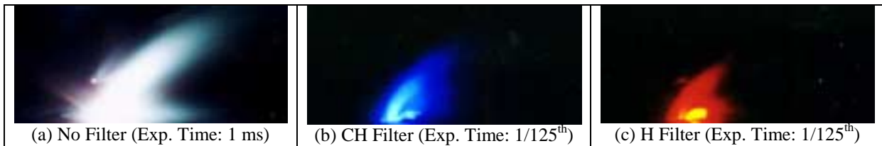
Figure 9.3: Filtered Photographs Showing the Effect of Aeroramp Lifting on Plasma Species ( P_t=2500 W, q_t=1.17 , q_{inj}=3.00 )
