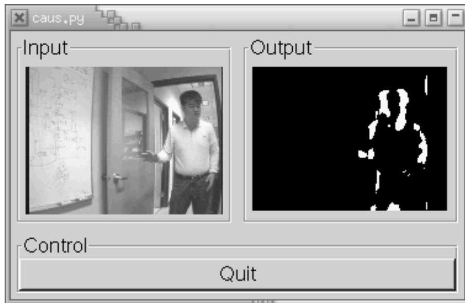
Figure A.4: Binary image generated by the motion detection algorithm demonstration
