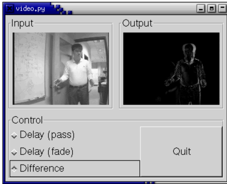
Figure A.3: Screen capture of video processing with the difference filter
