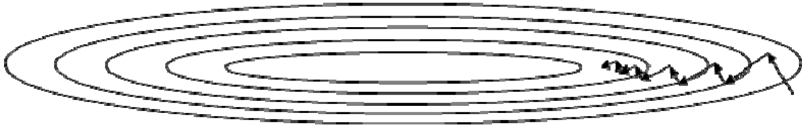
Figure 4.1: An example of a curve for which gradient descent would converge slowly.
