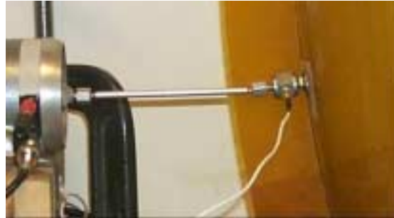
Figure 3.2. Electromagnetic shaker attachment to the skin of the torus.
