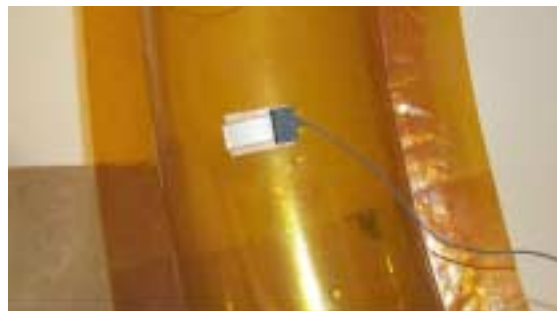
Figure 3.3. PVDF sensor attached to the skin of the inflated torus.
