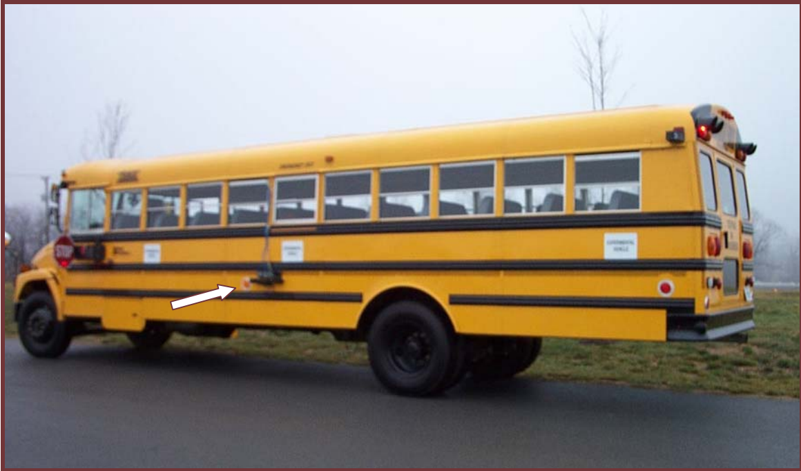
Figure 14. Violation recording cameras positioned in a central location.
