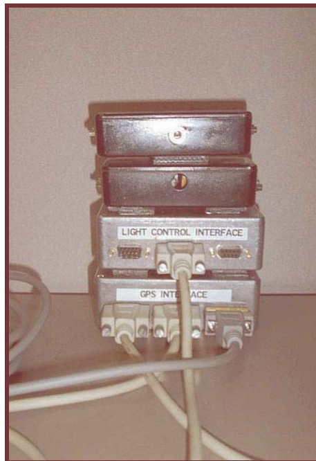
Figure 11. Four control boxes used in the prototype system.
