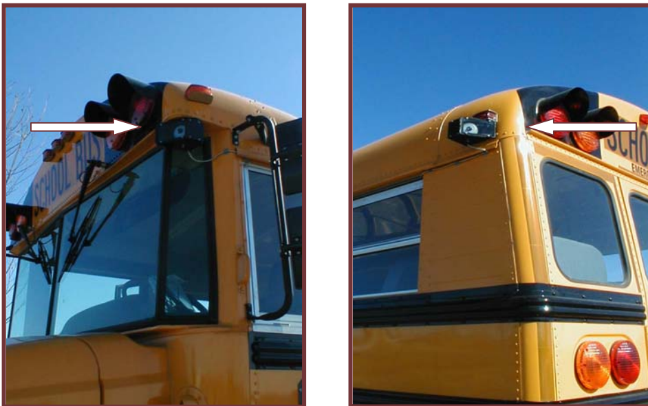
Figure 13. Violation detection cameras on front and rear of school bus.
