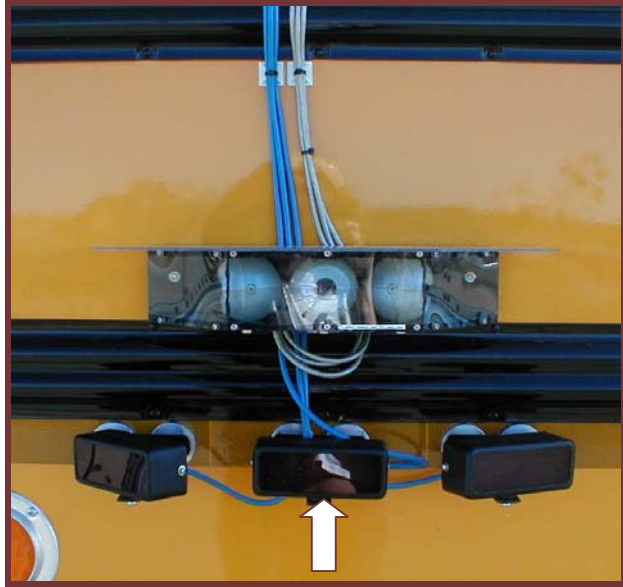
Figure 17. Three infrared pulse sources mounted on side of bus.
