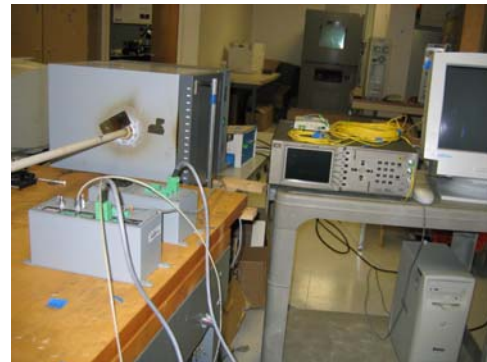
Figure 3-21. System setup for high-temperature static pressure test.
