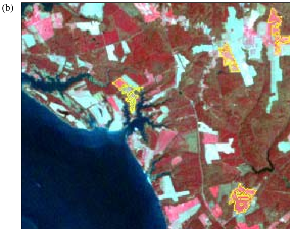
Fig. 2. Landsat TM multispectral image subset showing bands 4, 3 and 2 in red, green and blue, and training data areas of interest (AOIs) in yellow. The AOIs in (b) are a subset of those in (a).
