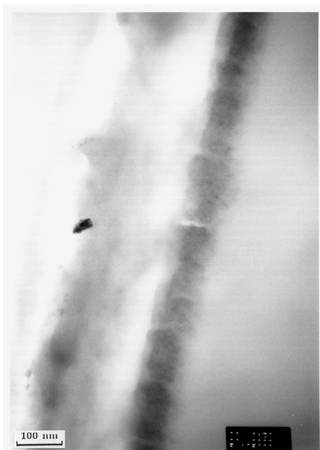
Figure 89 TEM image of an unheated P3OT/C 60 bilayer. The image shows two rather distinct layers. The C 60 has the darker contrast. There are no clusters of C 60 in the P3OT layer. This shows that diffusion of clusters of C 60 does not occur at room temperature or during sublimation of C 60 .
