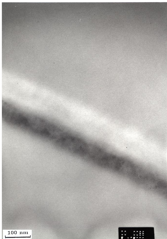
Figure 66 TEM image of an MEH-PPV/C 60 bilayer device heated at 150 °C for 5 minutes. The interface between MEH-PPV and C 60 is smooth and distinct. There is no indication of a large-scale interdiffusion of C 60 into the MEH-PPV bulk.
