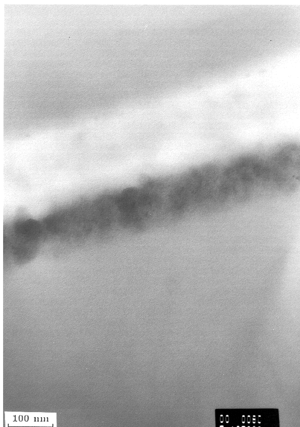
Figure 65 TEM image of an unheated MEH-PPV/C 60 bilayer. The light phase is MEH-PPV, the dark phase is C 60 and the gray background is from the epoxy. The picture shows a distinct and smooth interface between the two materials.
