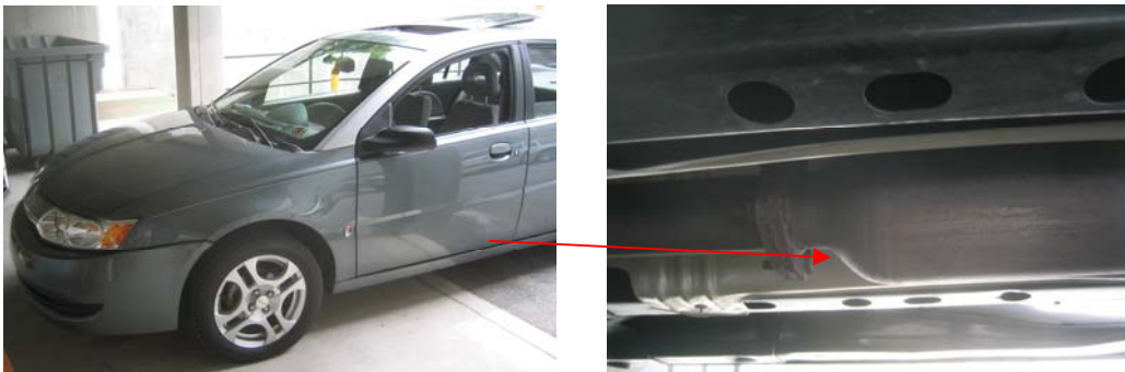
Figure 4.2.1. Photograph of automobile and mounting location of TEG device.
