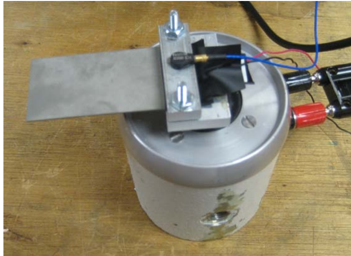
Figure 3.2.8. Photograph of test setup with Kistler teardrop accelerometer secured to the base.
