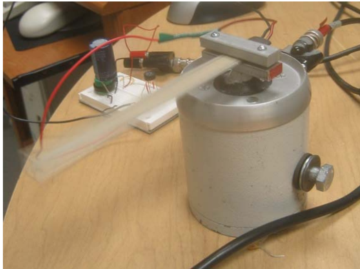
Figure 3.3.2. Photograph of AFC attached to the shaker, vibrating at its first natural frequency.
