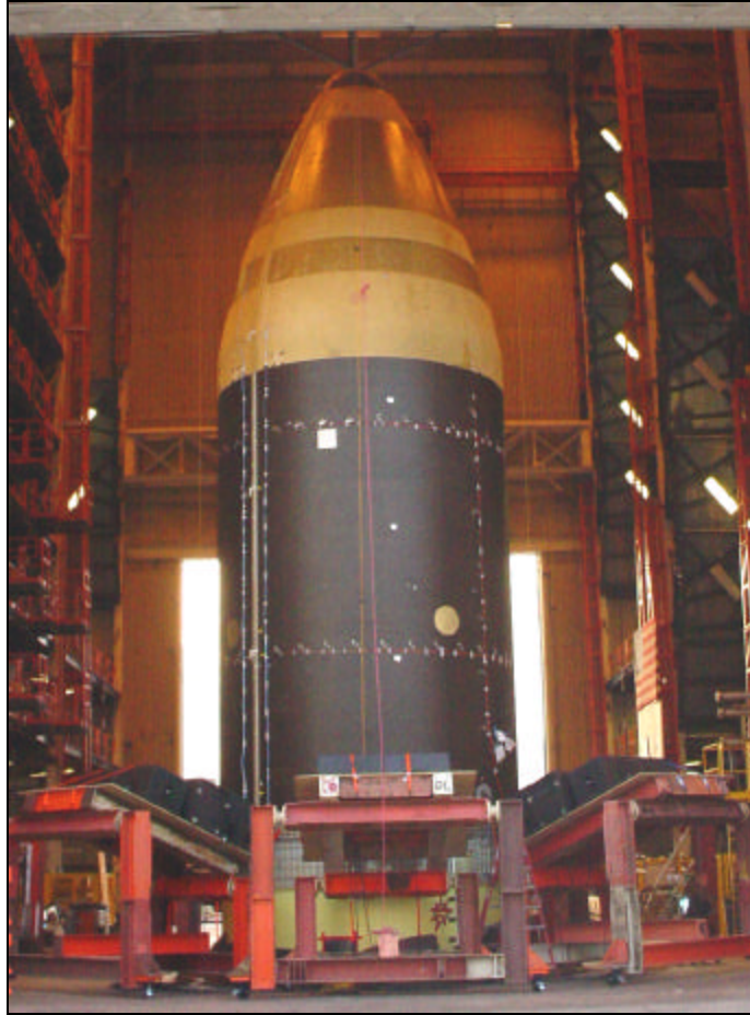
Figure 2-14. Picture of the test fairing together with the speakers providing external disturbance.
