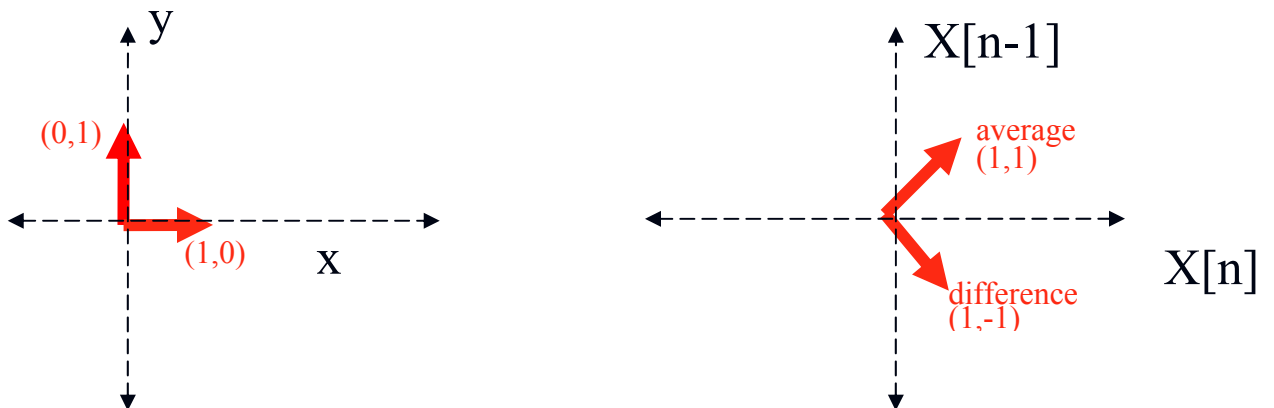
FIGURE 2-2: TWO BASES FOR THE TWO-DIMENSIONAL COORDINATE PLANE: (LEFT) STANDARD BASIS, AND (RIGHT) HAAR BASIS.
