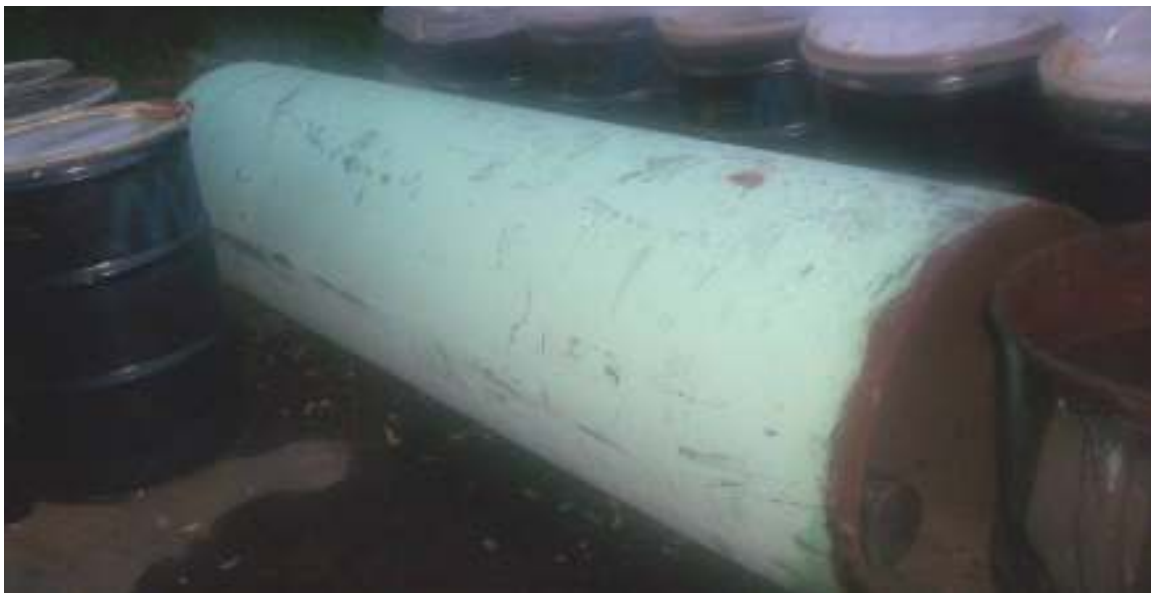
Figure 2.14. Pipe used to construct the pressure chamber (as received).
