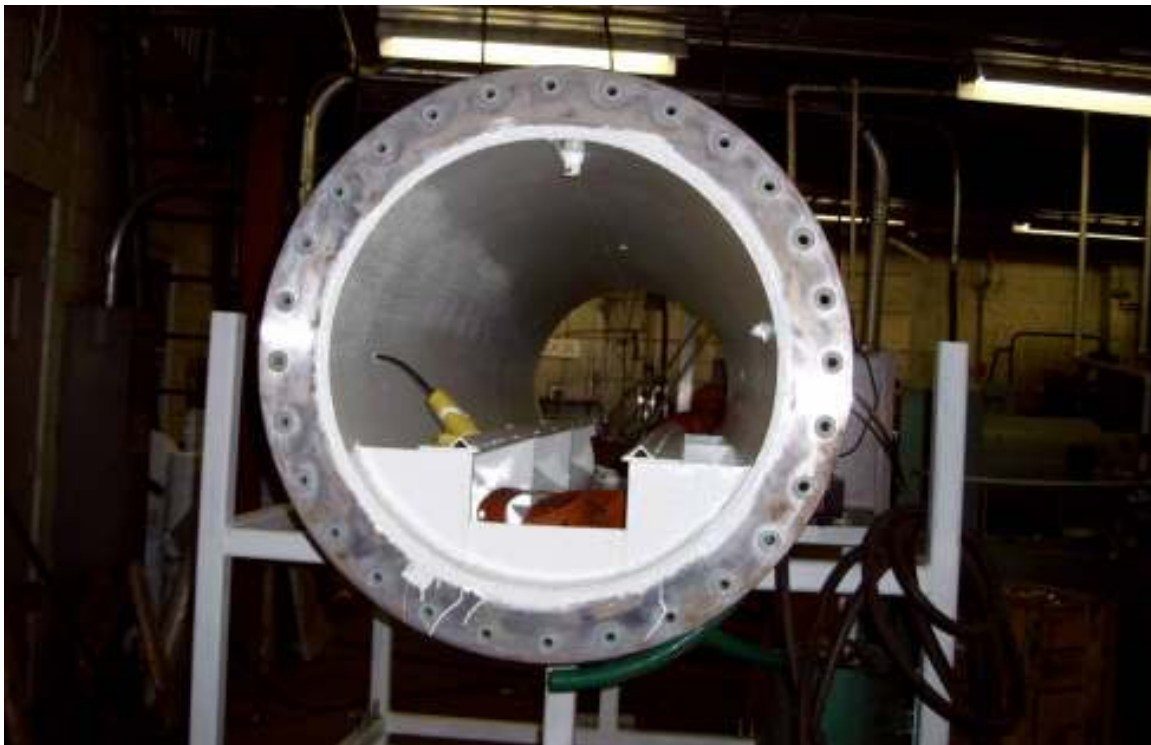
Figure 2.18. Flange attached to the ends of the pressure vessel.
