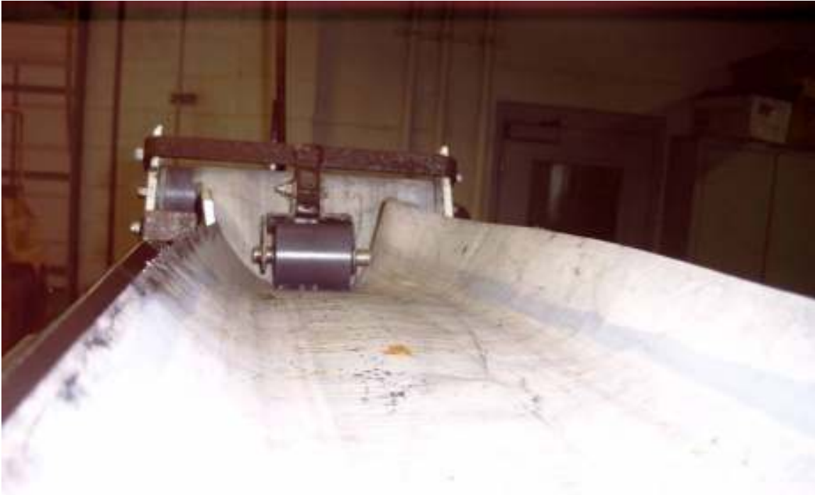
Figure 2.6. Trough apparatus used to hold slurry on the filter cloth.
