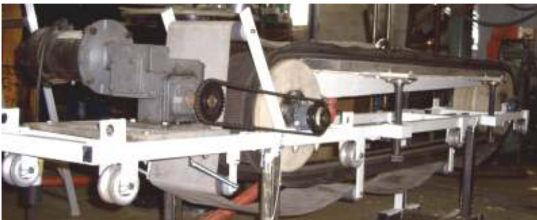
Figure 2.23. Completely assembled belt filter mechanism.
