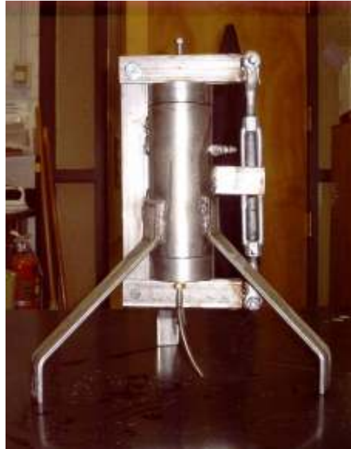
Figure 3.1. Batch pressure filter.
