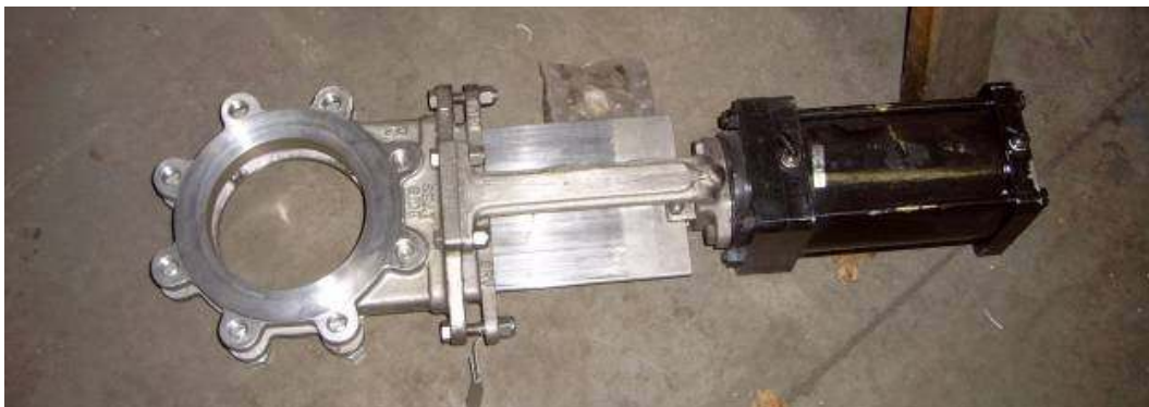
Figure 2.20. Knife gate valve used for the air-lock pressure seal.
