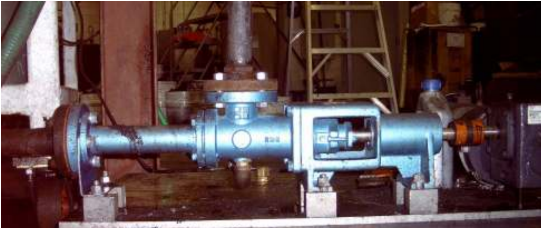
Figure 2.19. Progressive cavity pump used to feed the pressure filter.
