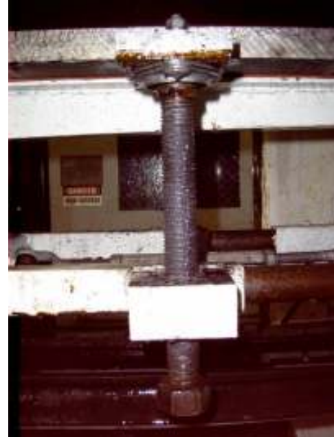
Figure 2.9. Bolts attaching frame to the pressure plate.
