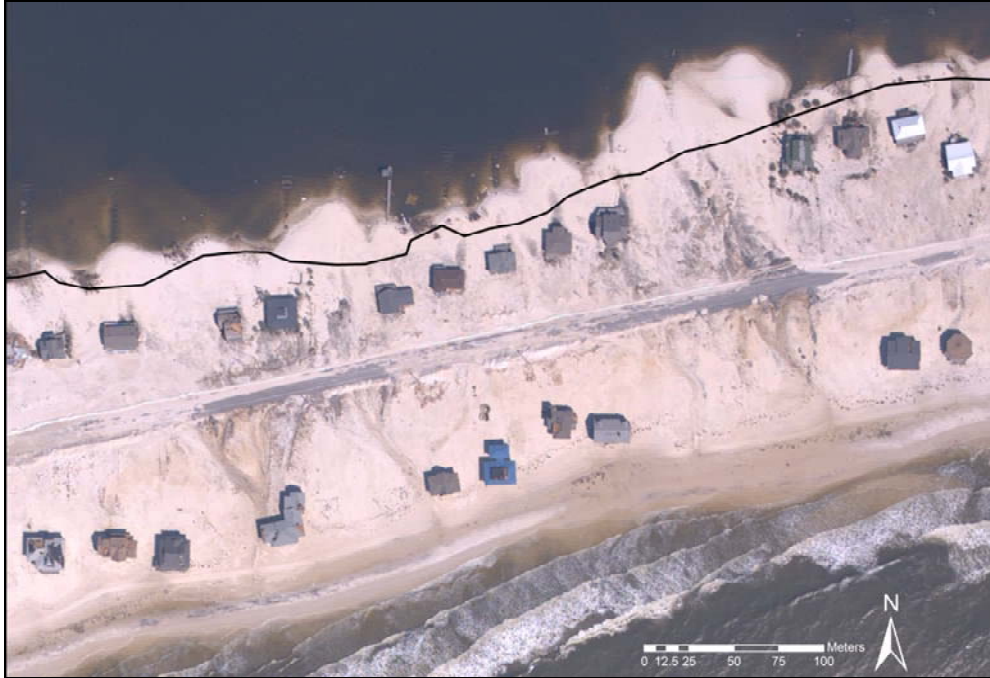
Figure 4-35 (Hurricane Ivan overwash fans in 2004, 1997 lagoon shoreline in black. Hurricane Ivan produced numerous overwash fans like those in this photo.)
