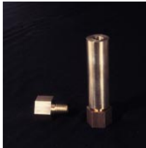
Brass bolts made on the lathe from hexagonal brass section.
