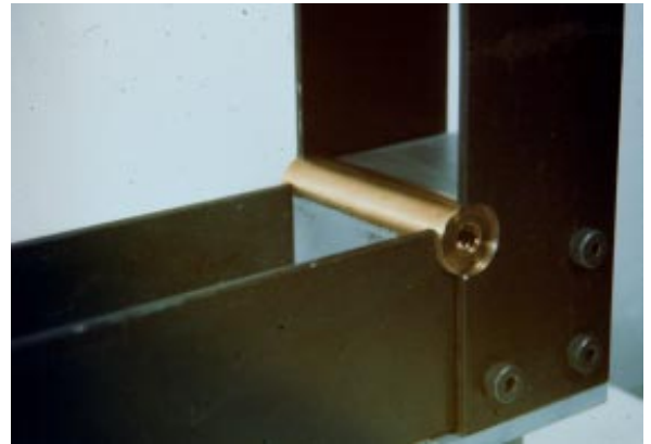
Aluminium cube as a support holds steel pieces and machine bolts keeps them together. Brass pin acts as a connector.
