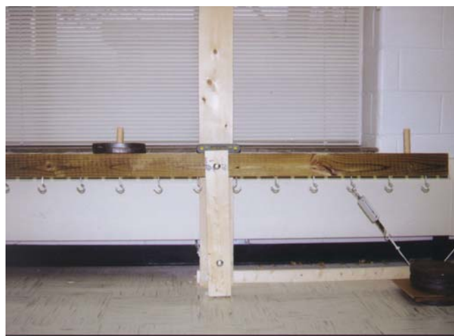
Figure 3: Lab 2, Exercise 2.2: The seesaw is made from a 4x4 piece of lumber. A small scale at the lower right side of the picture measures the reaction at an angle.
