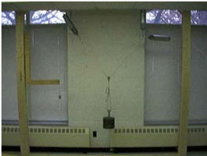
Lab 1, Exercise 1.2: The frame structure is built out of 2x6 lumber fastened by lag bolts. The rest of the equipment was purchased at a standard hardware or farm store.
