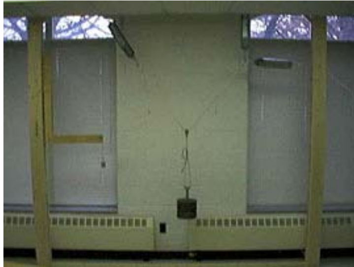
Figure 2: Lab 1, Exercise 1.2: The frame structure is built out of 2x6 lumber fastened by lag bolts. The rest of the equipment was purchased at a standard hardware or farm store.
