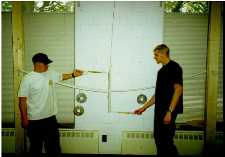
Figure 5: Two students demonstrate moment in Lab 5. The “beam” is made out of PVC pipe. There are actually two PVC beams: one behind, to which a moment is being imparted by two hanging weights, and one in front, which is cut in half so that students can measure the amount of force required to duplicate the curve of the pipe behind it.
