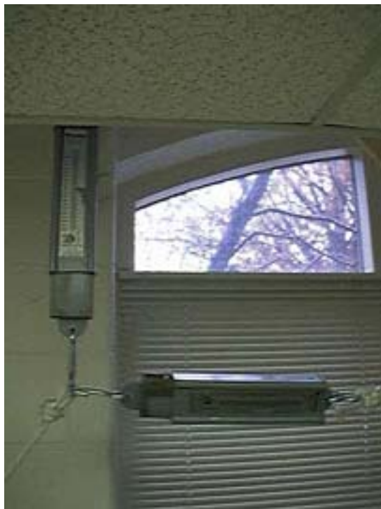
Lab 1, Exercise 1.2: Detail of how two scales were used to demonstrate reactions in both the x and y coordinates planes.
