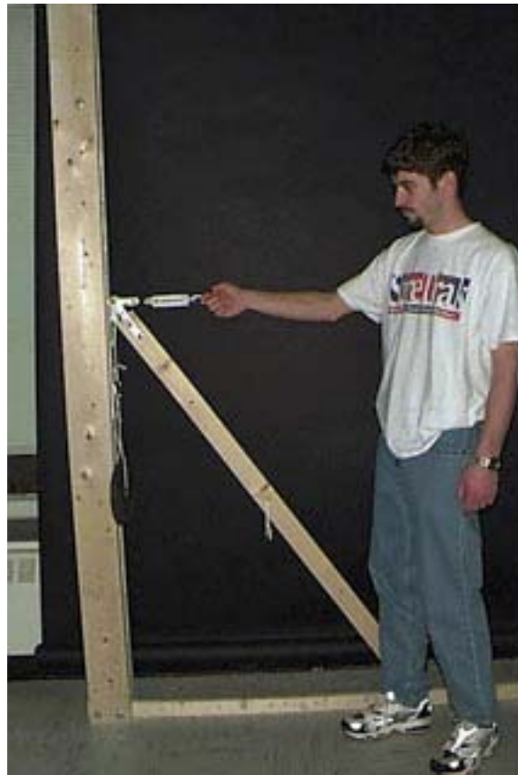
Lab 3: At the top of this member is a roller connection. At the bottom is a pin.
