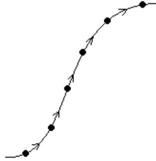
Figure 4.1 A path is approximated by a series of discrete configurations and their nominal paths.
