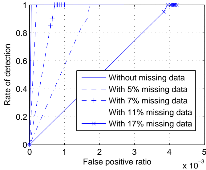
Figure 5.9: ROC curve for SYN Flood attack detection using varying degrees of missing data (via random sampling).
