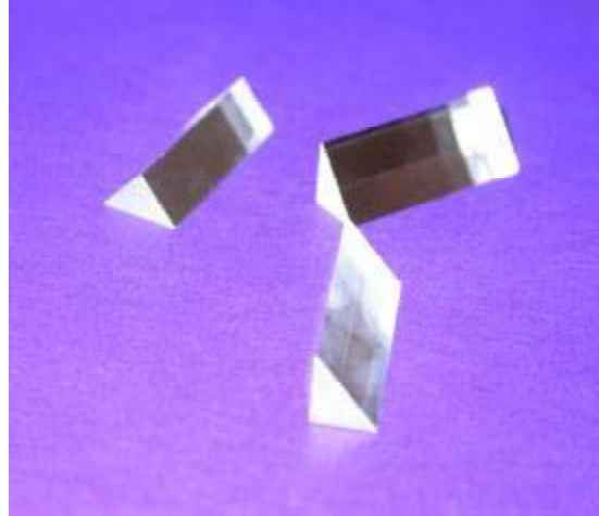
(b) Fabricated single crystal sapphire right angle prisms
