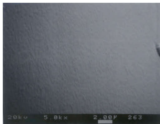
Figure 4.13. SEM of outside skin surface of non-terminated PET and PET-5%SSBA, 5.0K x
