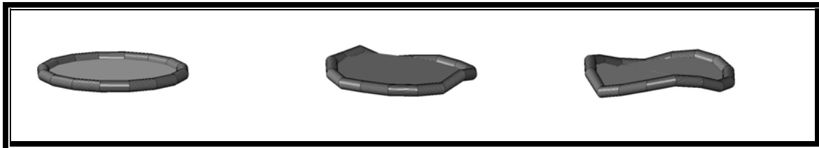
Figure 2.3: Experimentally identified mode shapes of an inflated torus with attached membrane mirror (pictured at top). The torus is shown at rest (left) and vibrating at the first and second out-of-plane modes (middle and right).
