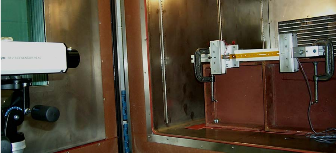
Figure 5.4. Photograph of the test setup, highlighting the laser vibrometer sensor and the Kapton sample test rig sitting inside of the Tenney Environmental vacuum chamber.
