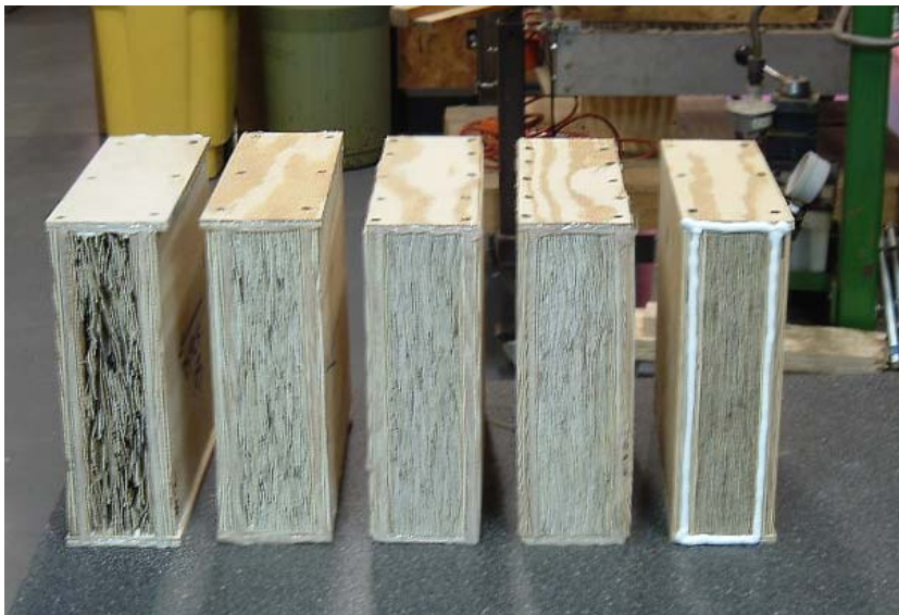
Figure 3-5. In-plane permeability specimens at all five density levels increasing from left to right.
