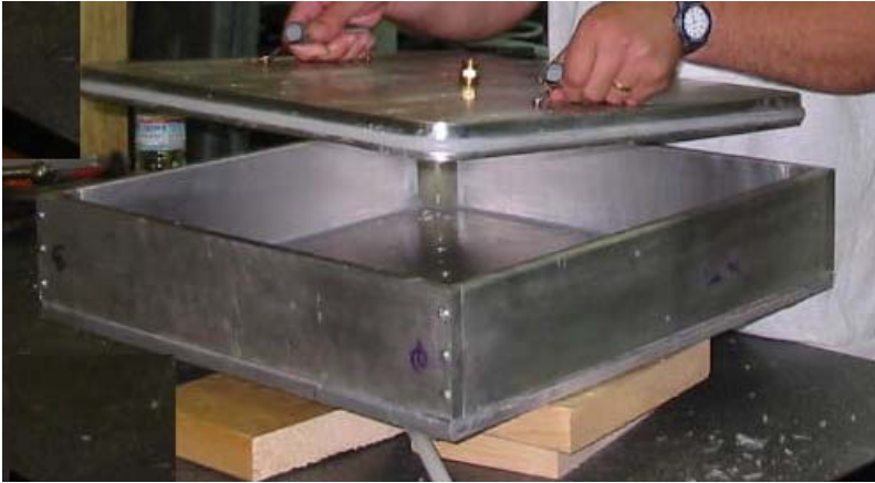
Figure 3-8. Transverse permeability specimen holder.
