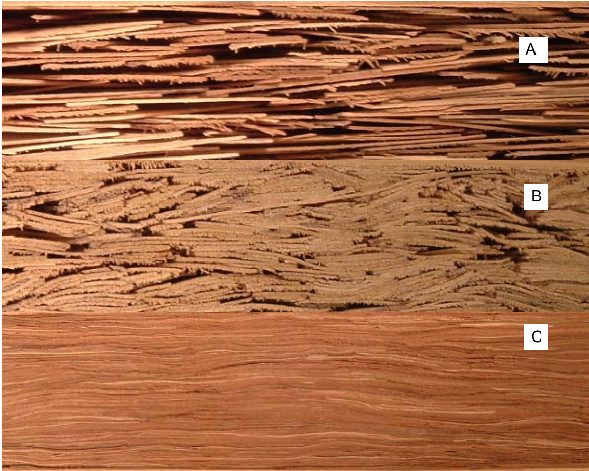
Figure 4-10. The progression from low to high compaction ratios. A. 0.28, B. 0.93, C. 1.48.
