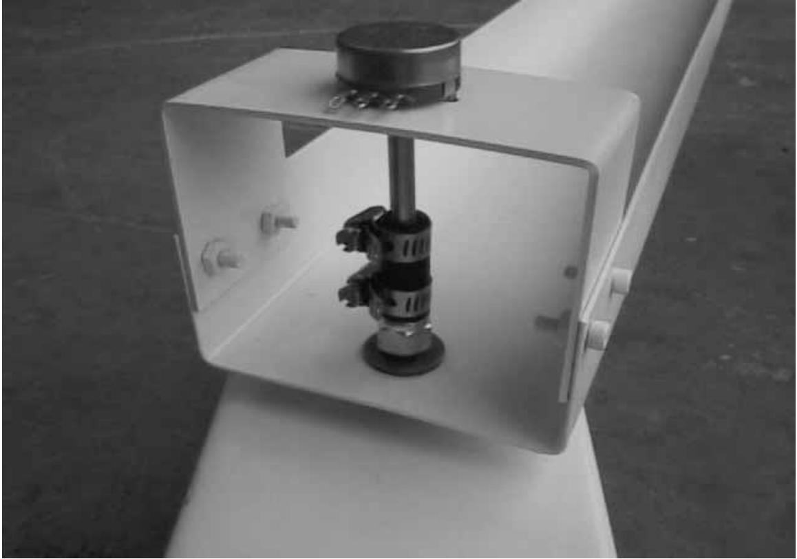
Figure 7. MBC/Pig Joint After Final Assembly
