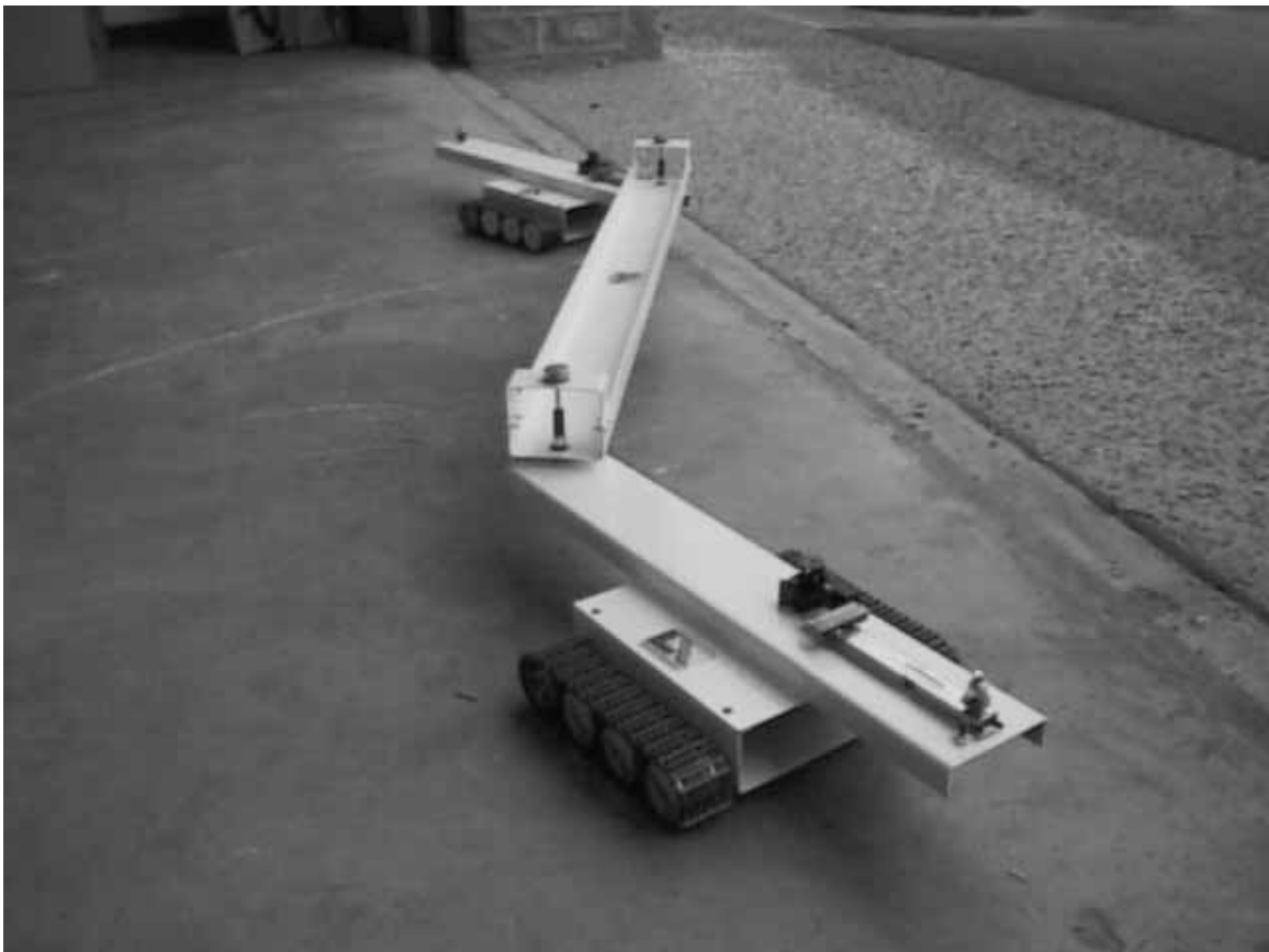
Figure 8. Prototype CHS Featuring Two MBCs and a Pig
