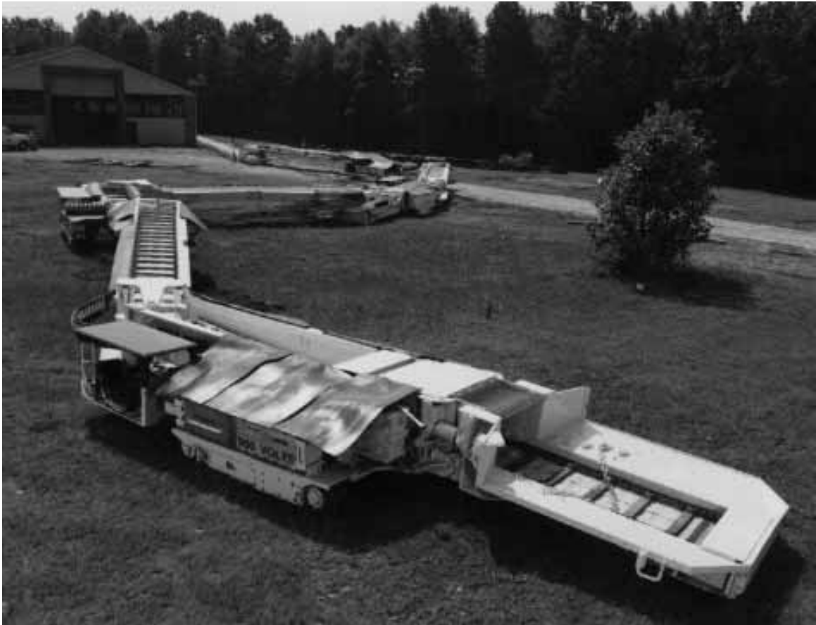
Figure 3. Continuous Haulage System used for VA Tech Team Test Driving
