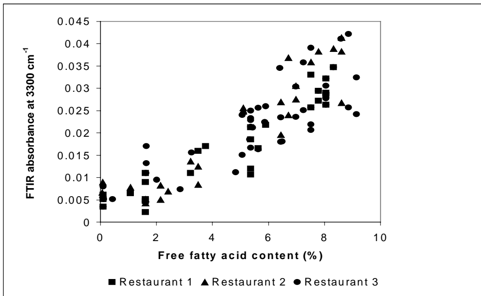
Figure 7.4 The correlation between chemical properties (PV and FFA) and FTIR absorbance.
