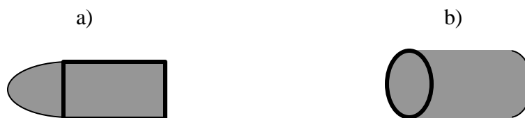
Figure 2.2. (a) Shows a standard 9mm bullet, (b) shows a blunt ended cylindrical bullet
