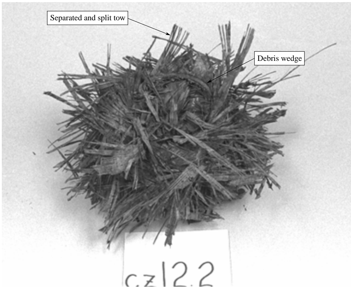
Figure 5-2: Splaying crush mode (with socking also seen)
