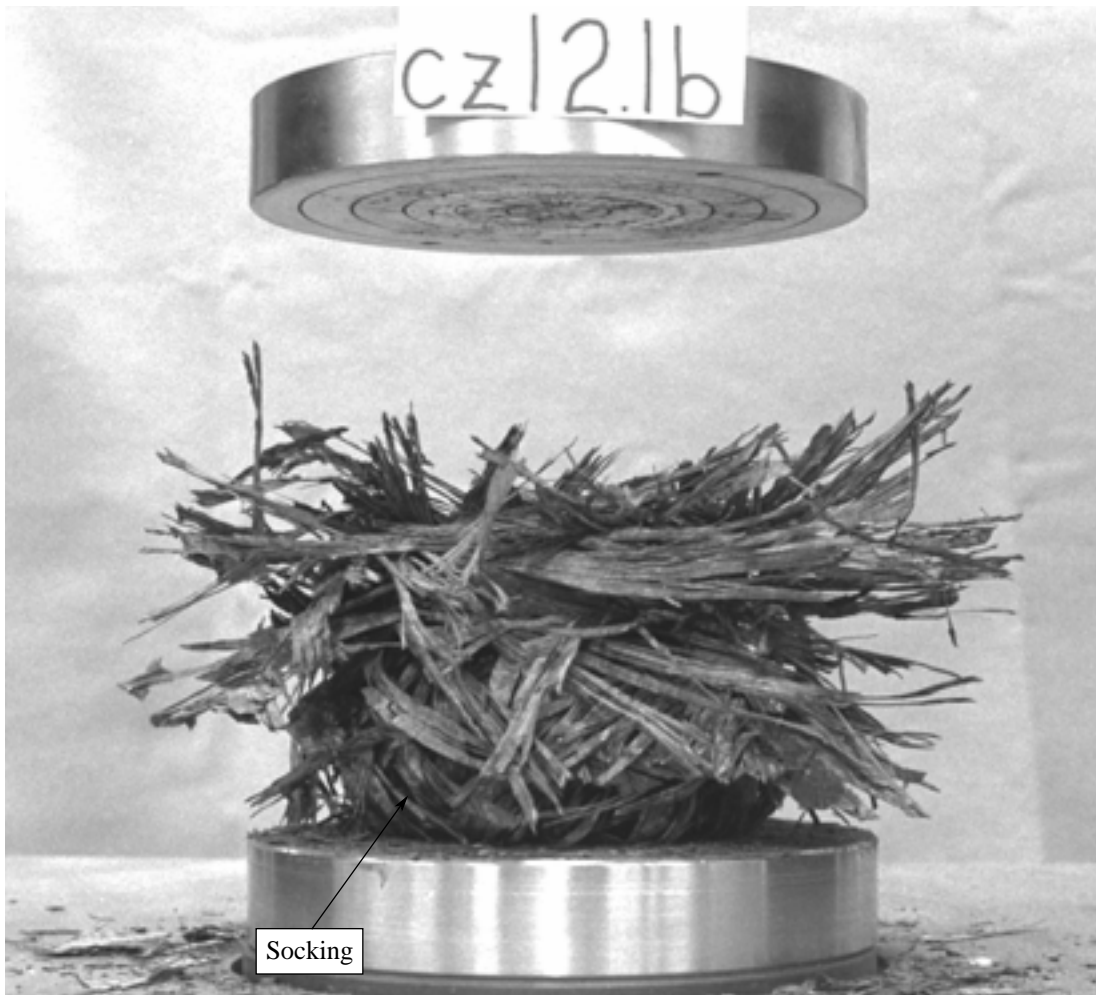
Figure 5-3: Socking crush mode (with splaying also seen)
