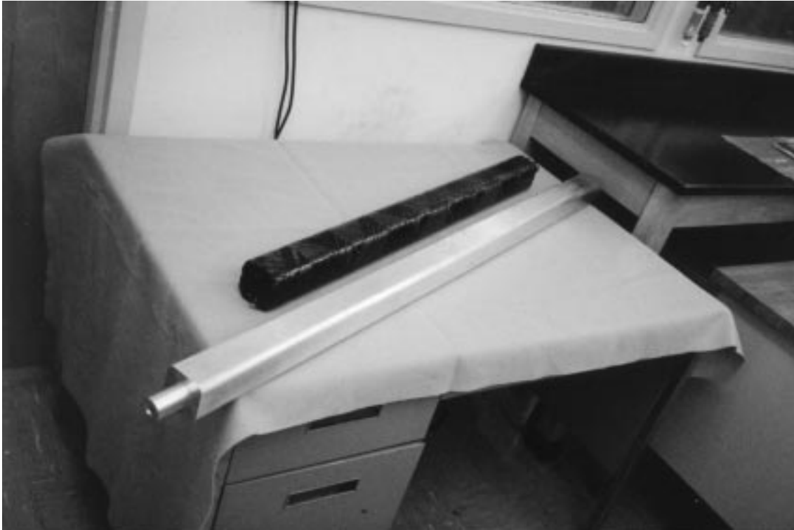
Figure 3-2: Aluminum mandrel used for filament winding the square tubes with uncut square tube
