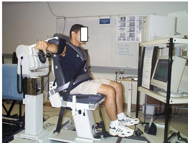
Figure 2.1 Participant posture for isometric shoulder abduction (right hand at horizontal position with feedback of exerted torque shown on a computer screen).
