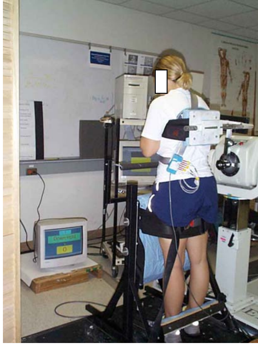
Figure 4.1 Equipment and fixtures for isokinetic torso extension (instructions shown on a computer screen).
