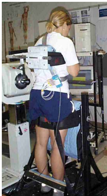
Figure 2.2 Participant posture for isometric torso extension (the lower body is stabilized using a fixture attached to a force plate).
