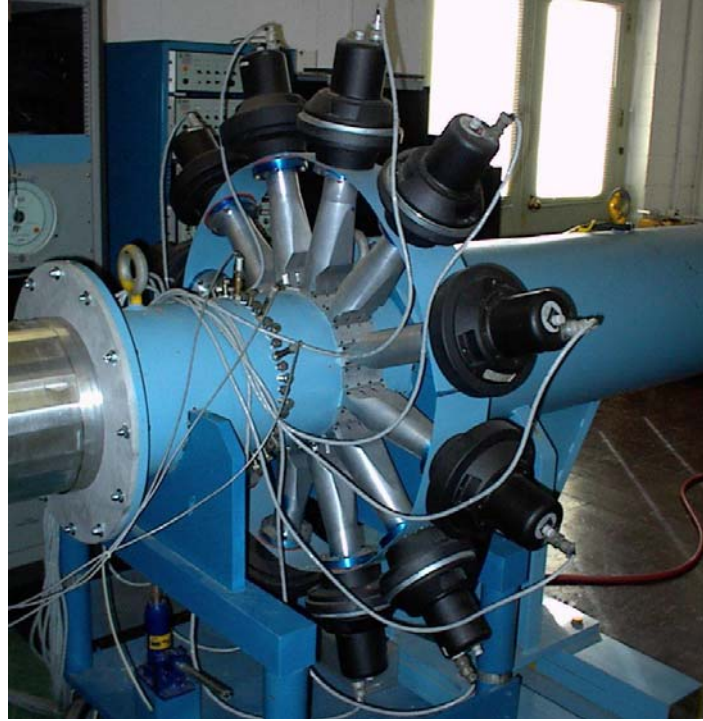
Figure 3-2: Array of 12 equally spaced acoustic drivers.
