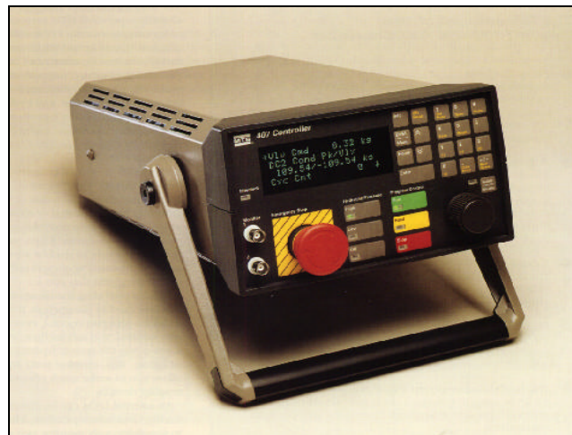
Figure 2.7 MTS Model 407 Servo Hydraulic Controller [31]
