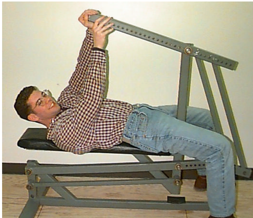
Figure 9-3, Prototype in the Pushing Configuration
