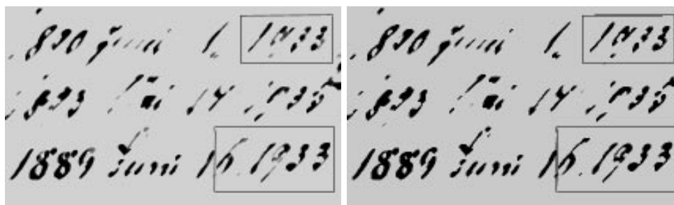
Figure 5.9: (Left) Result from the morphological closing. (Right) Result of contrast stretch and brightness adjustment applied to the figure on the left.
