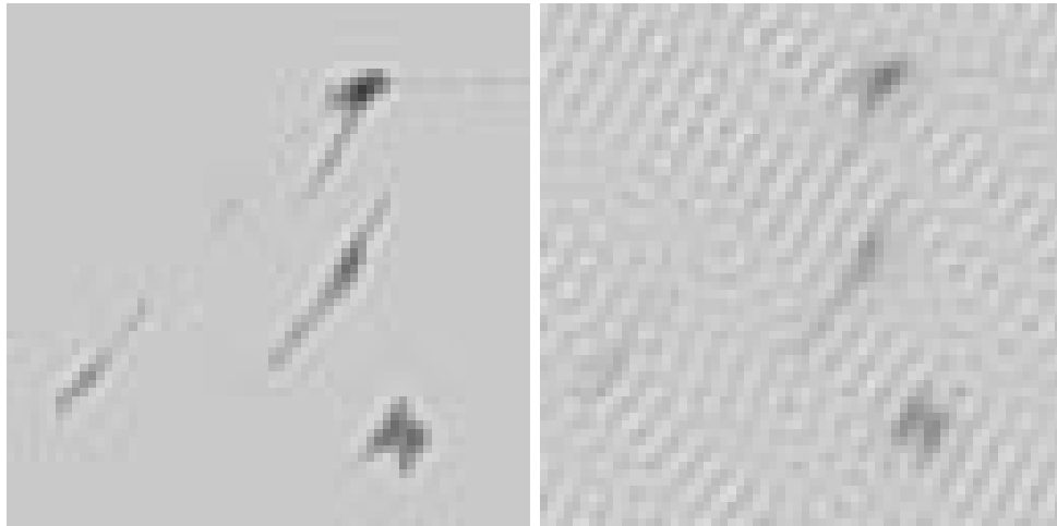
Figure 4.5: (Left) Sample image from the document library. (Right) Result of applying the inverse filter to the sample.
