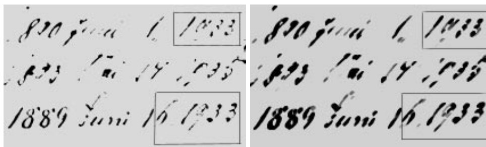
Figure 5.4: (Left) Result from the contrast stretch. (Right) Result of applying a gray level erosion to the image on the left.
