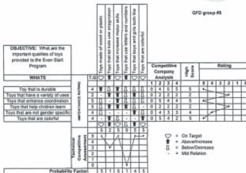
Figure 4. Quality functional deployment (QFD) chart.
