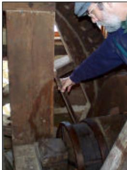
On return to the mill it will be necessary to disengage the stone. Remember to remove the safety wedge and then pull the wallower shaft out of gear (left). Remember to replace the safety wedge that goes behind the wallower shaft.
