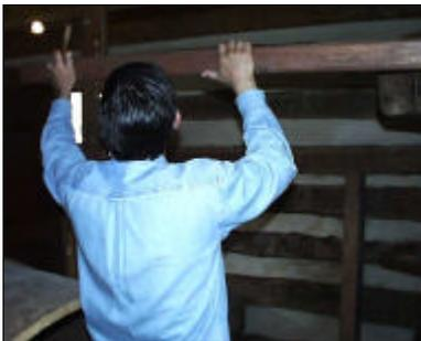
Use the lever inside the mill on the second floor to slowly open the gate over the wheel. Allow just enough water to start the water wheel turning. Once the wheel and stones are turning, examine the mill again. Check all the running parts on the first level. Make sure all things “look and sound right.” After some experience, one will be able to recognize unusual sounds during operation that may indicate a problem.
