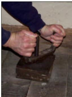
Start with a small amount of grain. Once the grain is between the stones, start lowering the stones. A clockwise turning of the screw (left) will lower the stones. As the stones get closer together, check your grind through the opening at the base of the vat. It may be now necessary to give the mill more water to sustain a consistent speed. The mill is now under a load and requires more power (water) to maintain an adequate grinding speed.
