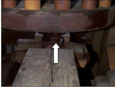
This adjustment is made on the first level of the mill by adjusting two wedges around the “trampot (arrow at left).” The trampot is the housing for the foot bearing of the millstone spindle. It is cast iron and sits on the bridge tree.
